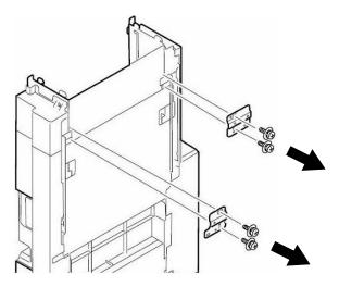
4. Turn the inverter around and remove the two screws holding the extension plate. Keep them handy to reattach the plate once it is repositioned.
